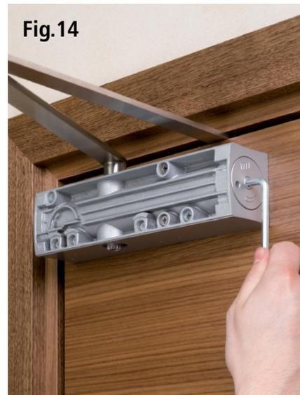
All Allgood door closer mechanisms are sealed for life and require little maintenance. However, a frequent check should ensure that the door closes freely and positively into the frame.
